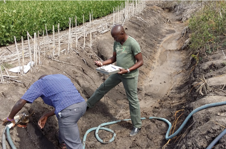
To improve water quality in heartland reservoirs, researchers at Iowa State University, Kansas State University, University of Missouri, and University of Nebraska worked with Extension specialists and farmers to develop gully erosion control practices. In the photo above, scientists test soil erodibility in a gully. Photo by Aleksey Sheshukov, Kansas State University.
